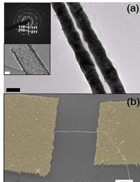
FIG. 1. (Color online) (a) TEM image of two 50 nm diameter Au-PZT core-shell nanowires, scalebar=50 nm. Upper inset, electron diffraction of a bundle of Au-PZT nanowires indexed as 110, 111, 210, and 211 of the perovskite form. Lower inset, empty 200 nm PZT nanotube, scalebar =50 nm. (b) SEM image of a single nanowire, scalebar=1  $\mu$ m.
