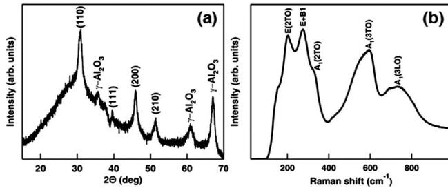
FIG. 2. (a), XRD of nanotubes within the AAO template. Indexed peaks are of tetragonal perovskite; all remaining indices are assigned to the AAO. (b) Raman spectrum of an individual 100 nm PZT nanotube in which the observed modes of tetragonal perovskite are denoted.
