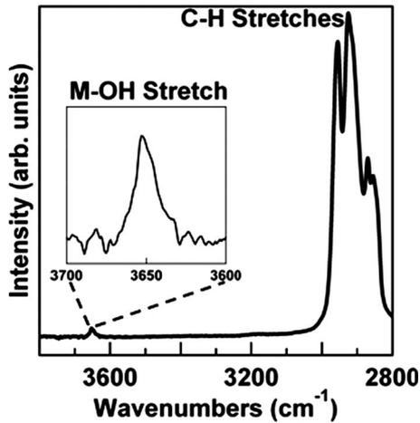
FIG. 4. FTIR spectrum of 100 nm PZT nanotubes. Inset shows an enlarged view of the 3650  $\text{cm}^{-1}$  peak, resulting from surface terminated hydroxyl species. The large peak at 2925  $\text{cm}^{-1}$  corresponds to C-H stretching modes.
