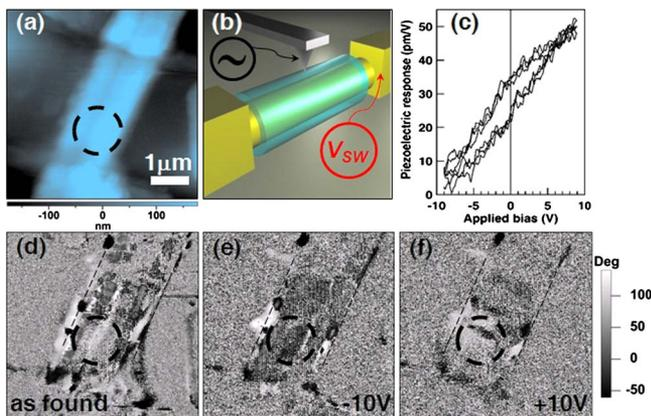
FIG. 3. (Color online) (a) Height map of a 100 nm Au-PZT coaxial nanowire. (b) Experimental scheme for collecting (c) FE piezoelectric hysteresis and (d)–(f) plane-normal piezoresponse phase contrast maps. (d) represents the “as-found” state with (e) and (f) revealing written negative and positive FE domains, respectively (dashed circles).
